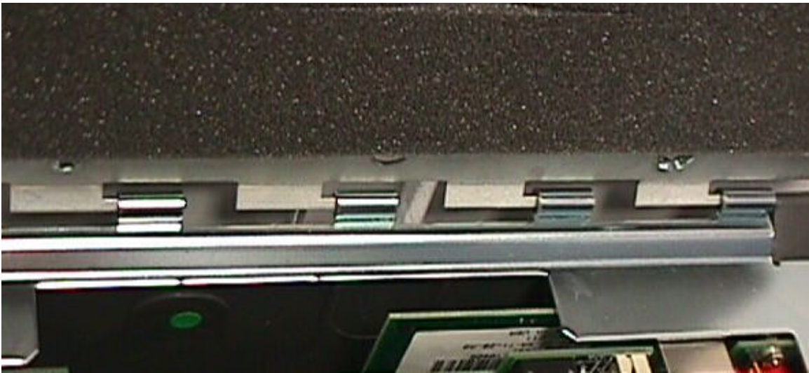
Figure 2B: Attaching the Hand Reader to the Wall Plate
